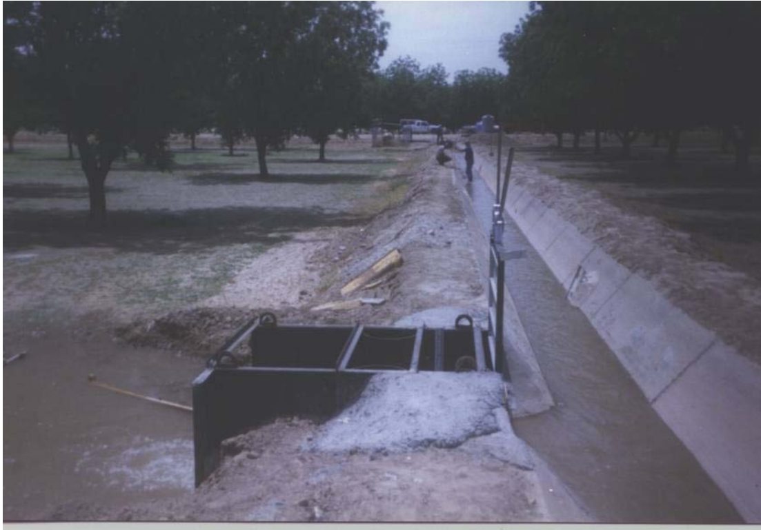
Fig. 4. S-M flume installed in turnout on a pecan farm in Southern New Mexico.
