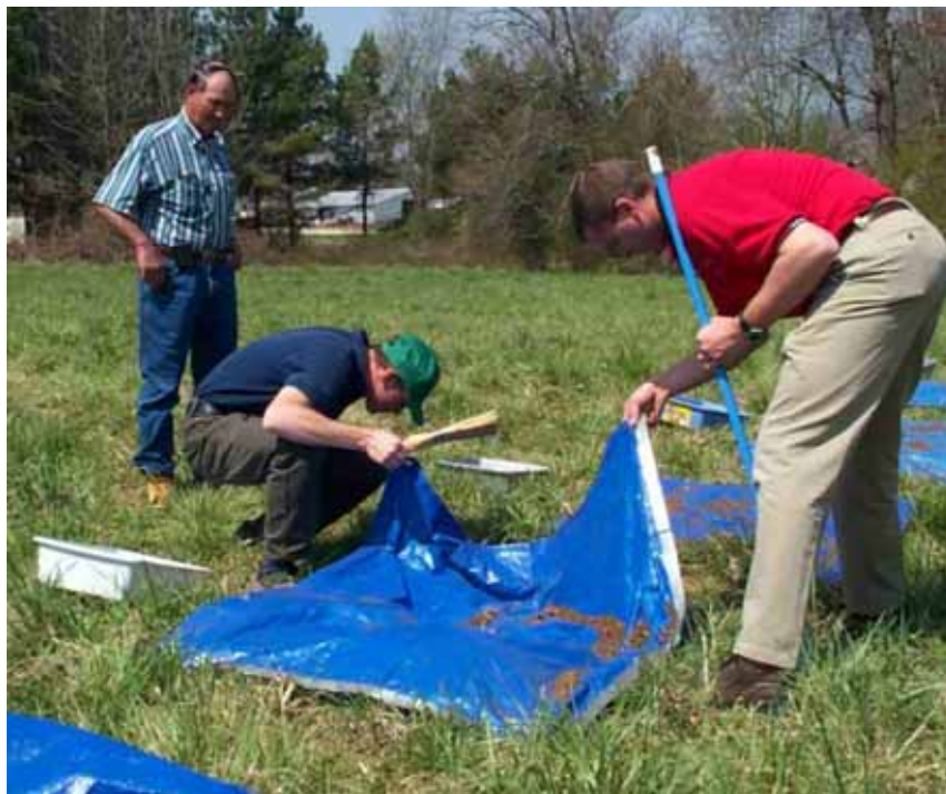
Figure 1. University of Georgia personnel using the small tarp method for poultry litter spreader calibration
