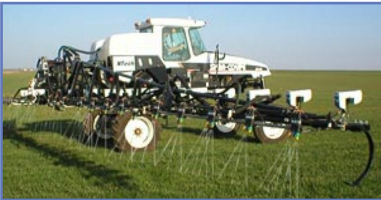
*Figure 1. Variable Rate (2x2 feet resolution) Green Seeker with multiple sensing units for site specific N application.*
