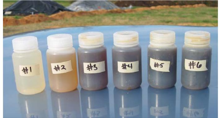
Figure 1. Contaminated runoff was obvious in all the uncovered piles. Runoff from the covered piles also appeared contaminated from litter spilled around the cover but the N and soluble P from the covered piles was much less than that from the uncovered piles. (#1= check plot/no litter; #2= 6-mil poly covered; #3=HayGard® covered; #4= uncovered; #5=cone-shaped pile; #6=polymer-coated pile)
