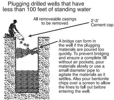
Figure 2. Plugging a well with bentonite chips.
