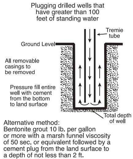
Figure 3. Plugging a well with a tremie tube.
